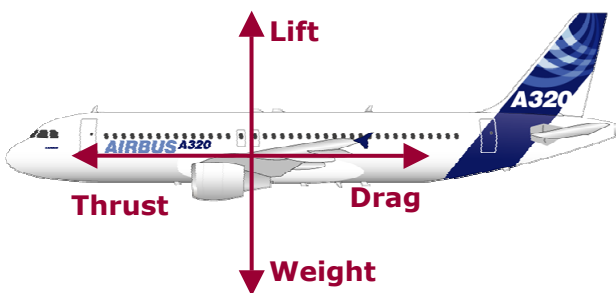
Figure 2-1 Elementary forces on an airframe
